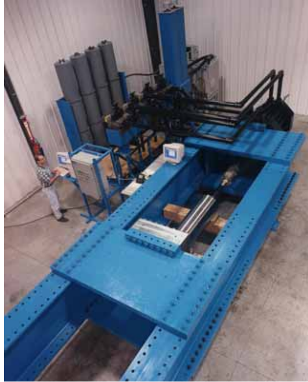
FIGURE 9 TAYLOR DEVICES' LARGE HYDRAULIC SEISMIC TEST MACHINE
