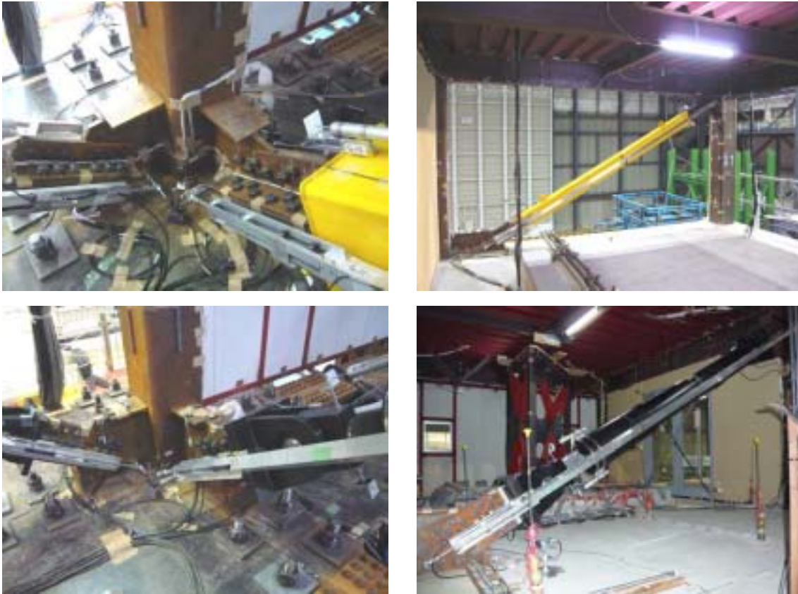
Figure 9. Measurement system of damper stroke and displacement of whole damper brace (Feb. and Mar. 2009)
