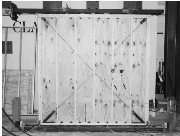
Figure 22. Experimental testing arrangement for wood-framed shear wall with hysteretic dampers along diagonals. (From Higgins 2001, © American Society of Civil Engineers. Reproduced with permission.)
