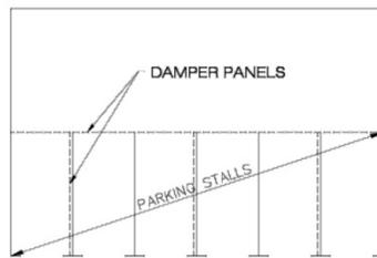
**Figure 3.** Plan view showing possible damper panel installation
