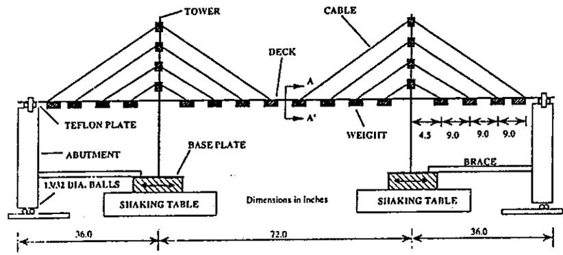
Figure 7. Configuration and dimensions of bridge model in experimental study
