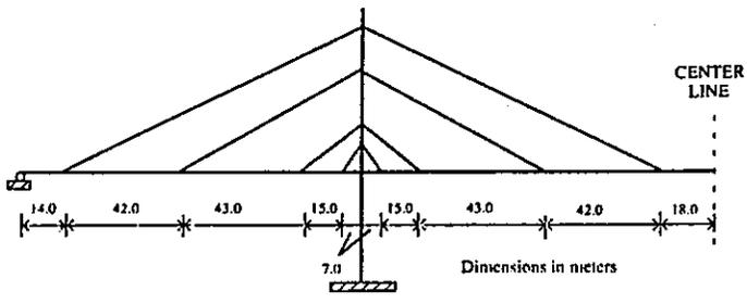
Figure 4. Elevation of bridge model in simulation study
