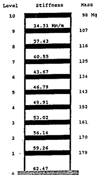
Figure 1. Ten-story shear building in numerical study
