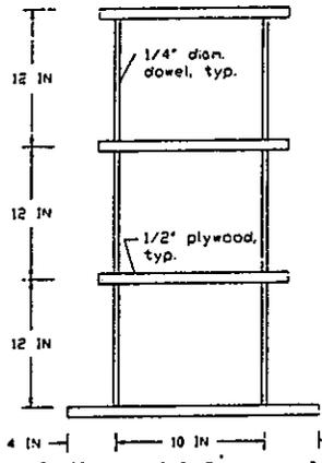
Figure 5. Building model in experimental study
