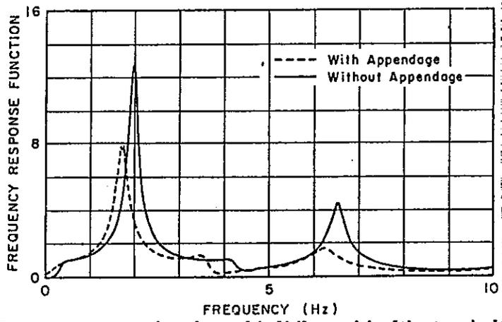
Figure 6. Frequency response functions of building model without and with damper
