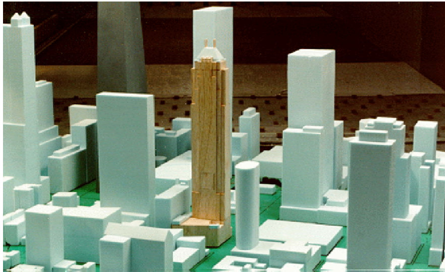
FIGURE 2 – MODEL OF THE PARK TOWER IN RWDI'S WIND TUNNEL
