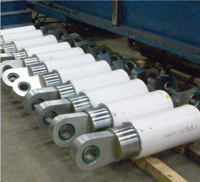
Assembled dampers ready for testing at Taylor Devices' North Tonawanda, New York, facility
