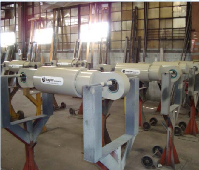
Dampers being painted prior to packing and shipping at Taylor Devices' Kenmore, New York, facility
