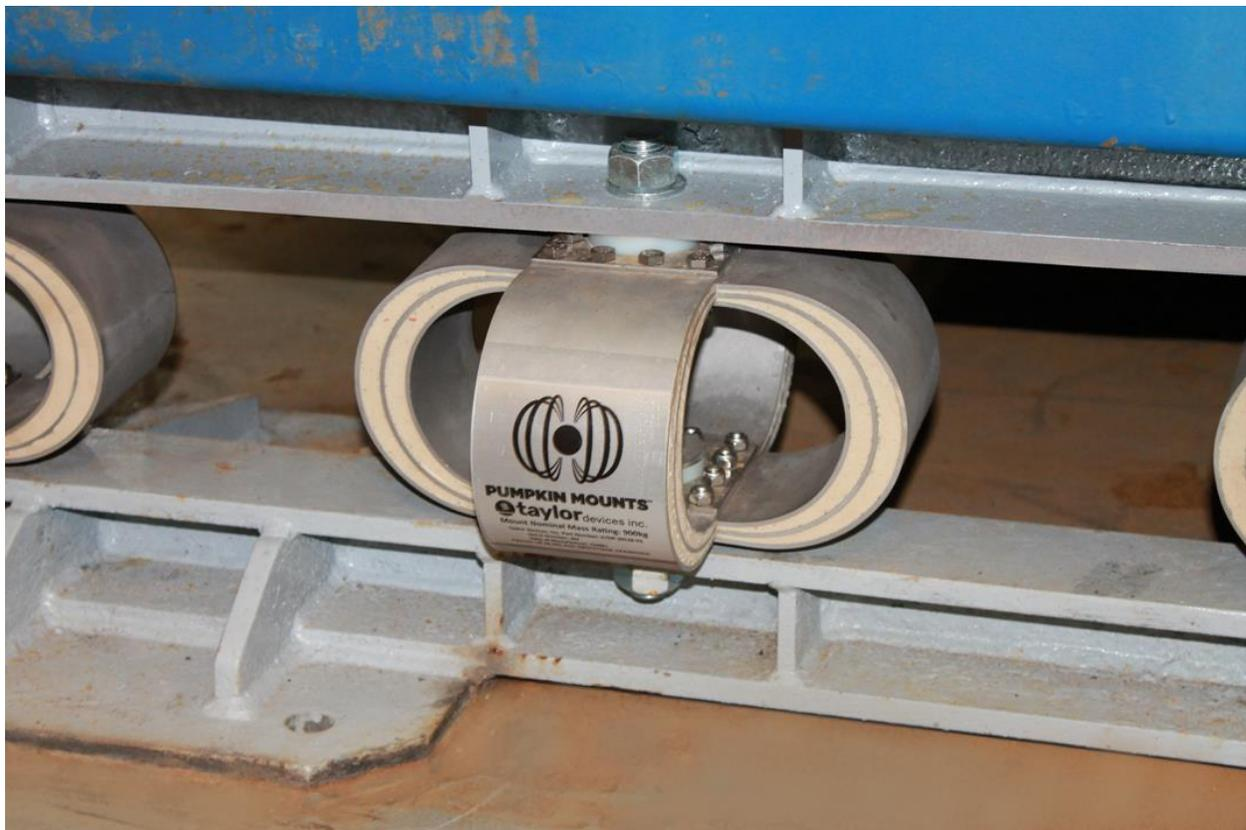
*1 Pumpkin Mounts installed just prior to shock testing*
