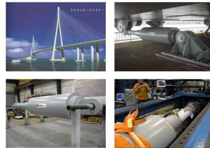
Fig.4 Sutong Bridge and dampers
