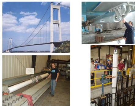
Fig 5 Jiangyin Yangtze River Bridge and dampers
