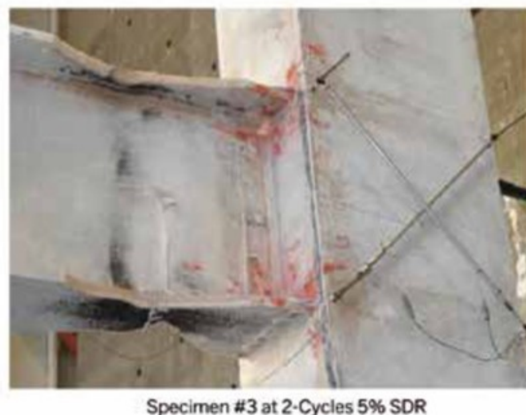
Figure 6. SMF Specimen #3 test results (UCSD).
