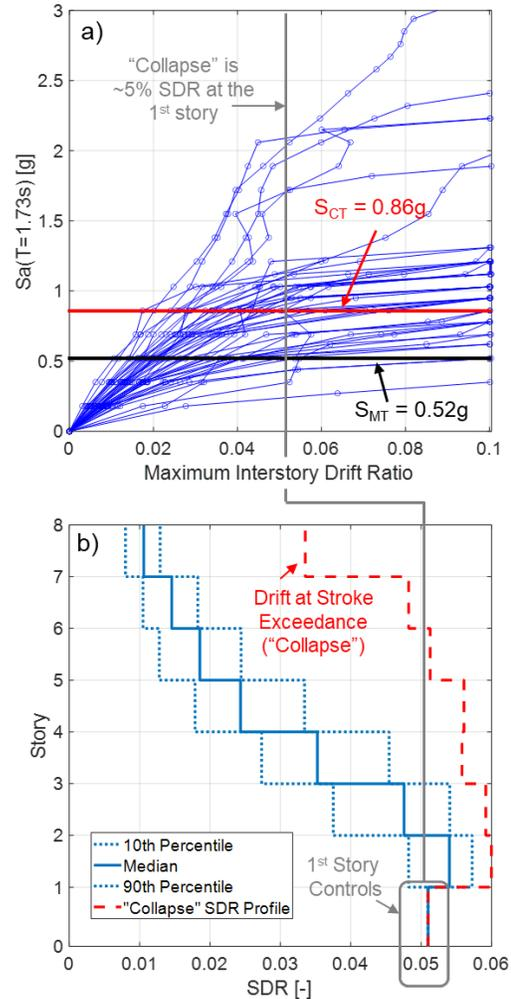
**Figure 7. a) Example IDA curves for an 8-story archetype, b) Story drift ratio profile corresponding to damper stroke exceedance (dashed red) compared with median response conditioned on stroke exceedance (solid blue). The gray line between the figures highlights that stroke exceedance governs collapse rather than a full sidesway mechanism**
