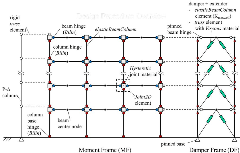
Figure 6. Nonlinear numerical model for a Type I TDMF™ system
