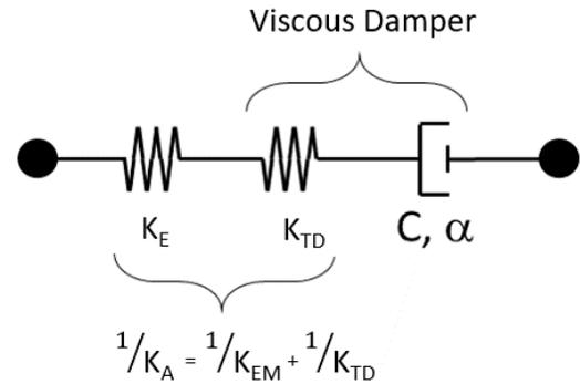
**Figure 5. Maxwell model used for modeling nonlinear viscous dampers**
