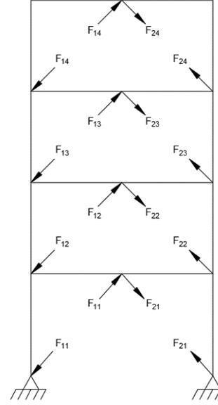
**Figure 2. Damper overstrength forces used for simplified analysis of a one-bay chevron damper frame**
