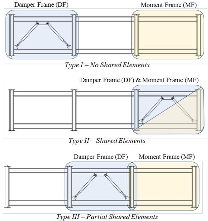
**Figure 3. Illustration of different TDMF™ system types**
