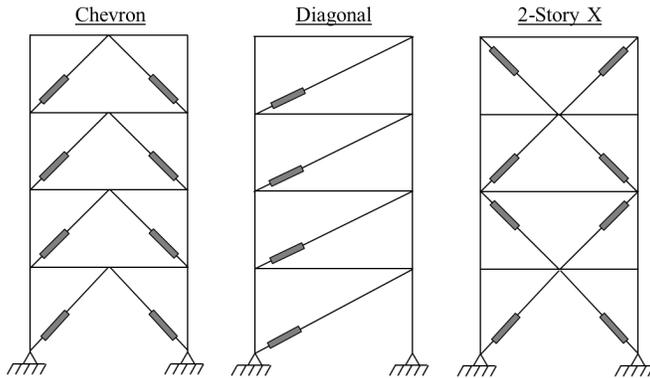
**Figure 4. Different damper configurations considered in the archetype design space**
