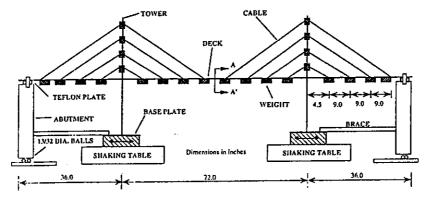
Figure 7. Configuration and dimensions of bridge model in experimental study
