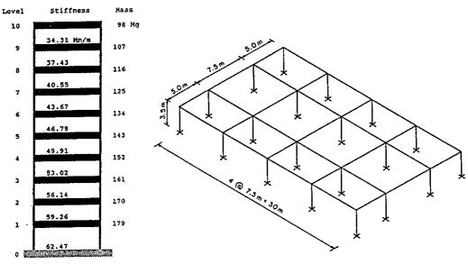
Figure 1. Ten-story shear building in numerical study
