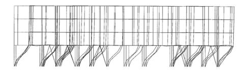
ETABS6.0 - Deformed Shape Elevation (Mode 1)
