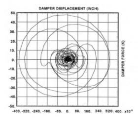
2nd Floor Displacement vs. V.D. Force
