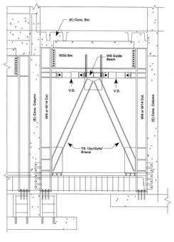
Typical VD Assembly Elevation G. Parker
