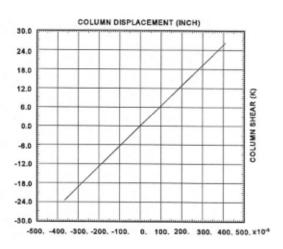
2nd Floor Displacement vs. Column Force
