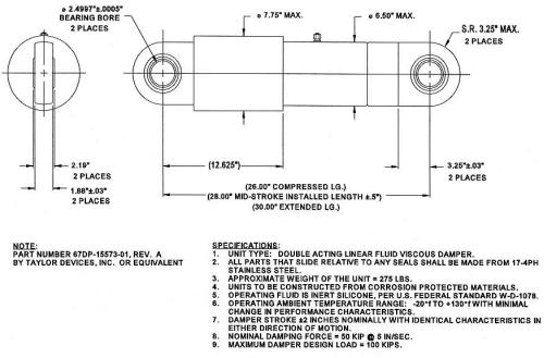
**Double Acting Linear Fluid Viscous Damper**
