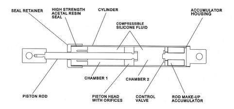
**Construction of Fluid Viscous Damper**
