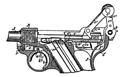
FIGURE 4 TOGGLE BREECH MECHANISM – MODEL PO8 LUGER PISTOL
