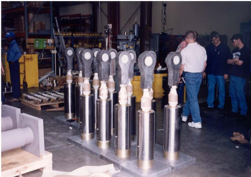
FIGURE 29 SAN FRANCISCO CIVIC CENTER DAMPERS READY FOR FINAL PAINTING
