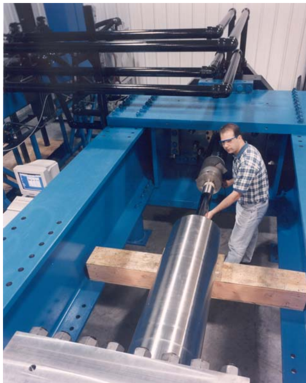
FIGURE 35 TESTING ON A DAMPER CARTRIDGE FOR THE PACIFIC NORTHWEST BASEBALL STADIUM
