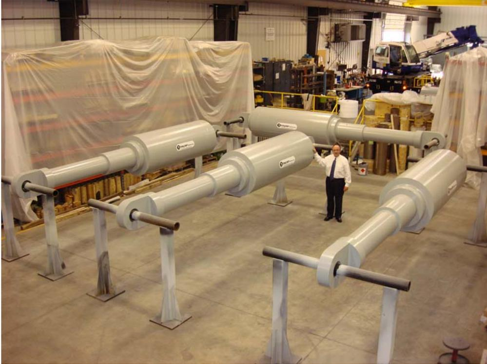
**Figure 13 – Completed Isolators**
