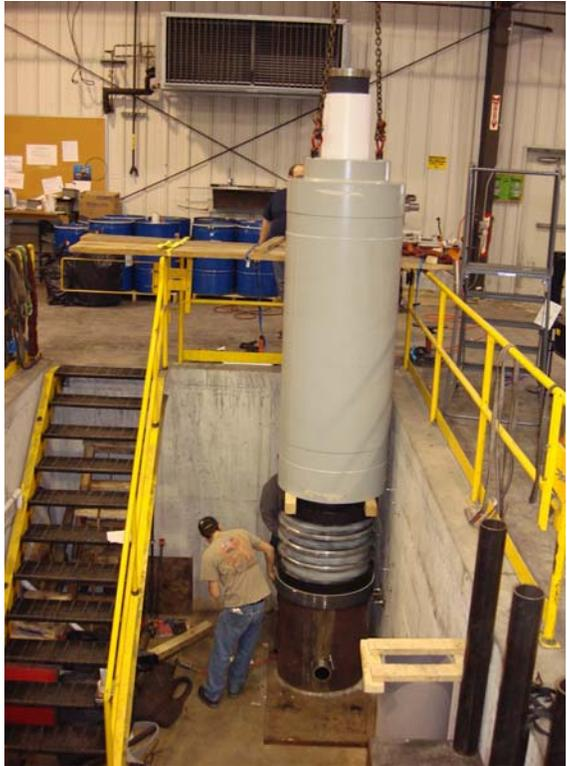
**Figure 12 – Subassembly of Spring Elements**
