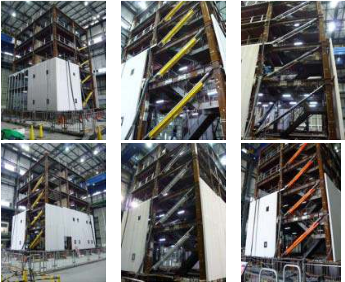
Figure 7. Four types of damper inserted in the building specimen (Feb. and Mar. 2009)
