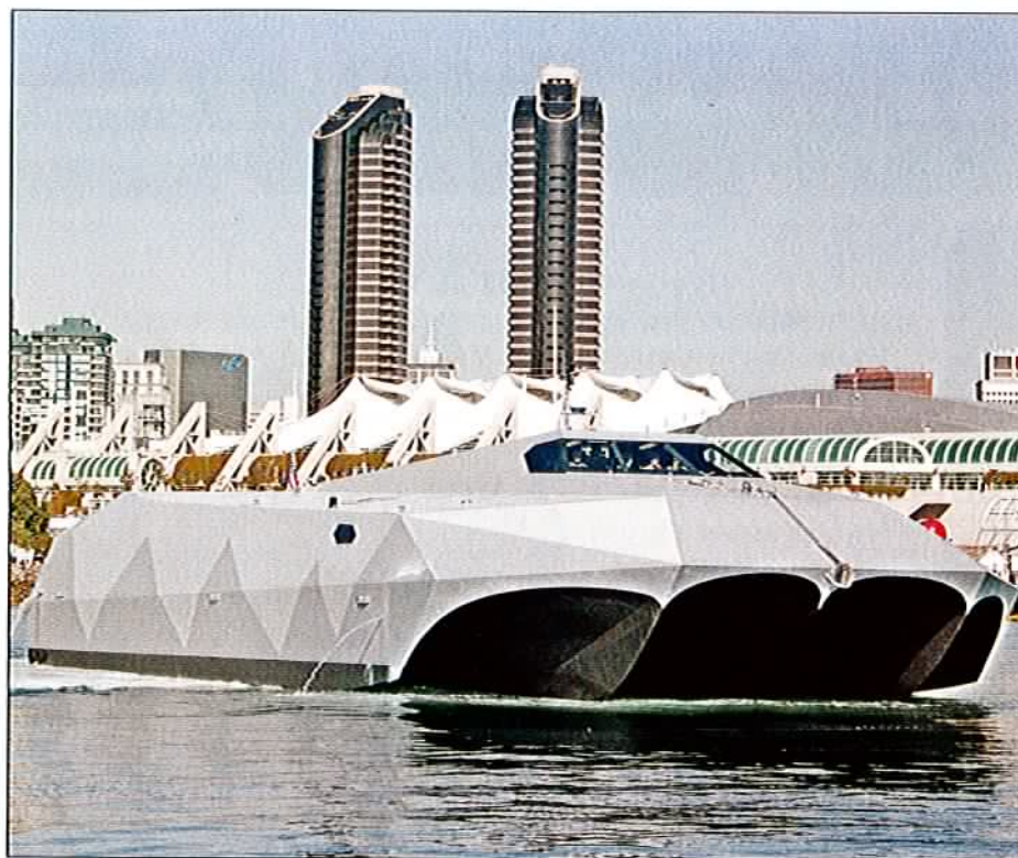
The M 80 Stiletto's hull design recaptures the bow wave using its energy to create an air cushion for more efficient planing. (Photo courtesy of M Ship Co.)
