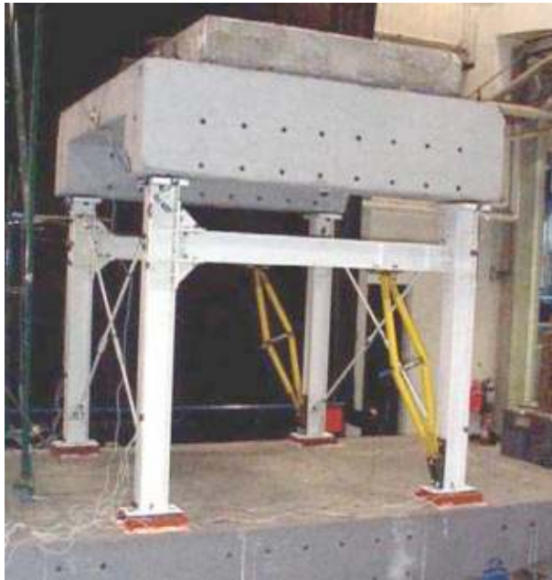
Figure 6. Model with scissor-jack damping system on the Buffalo earthquake simulator.
