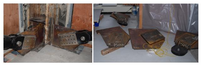
The gusset plates and tang plates may also be dimensionally adjusted and cut by the steel fabricator to provide the correct geometry, as they are simple and easy for the fabricator to customize.
